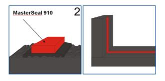
It is important to leave the minimum coverage from both the edges of concrete to provide sufficient concrete cover to absorb the swelling stresses.
