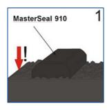
For normal joints width of 200-400 mm, place the waterbar along the middle of the joint. On wide joint surfaces (greater than 100 cm), two parallel waterbars may be laid for added safety.
